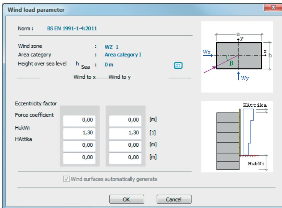
The wind loads are generated with consideration to the defined geometry and the border conditions specified in this dialog (Wind to x / y).
