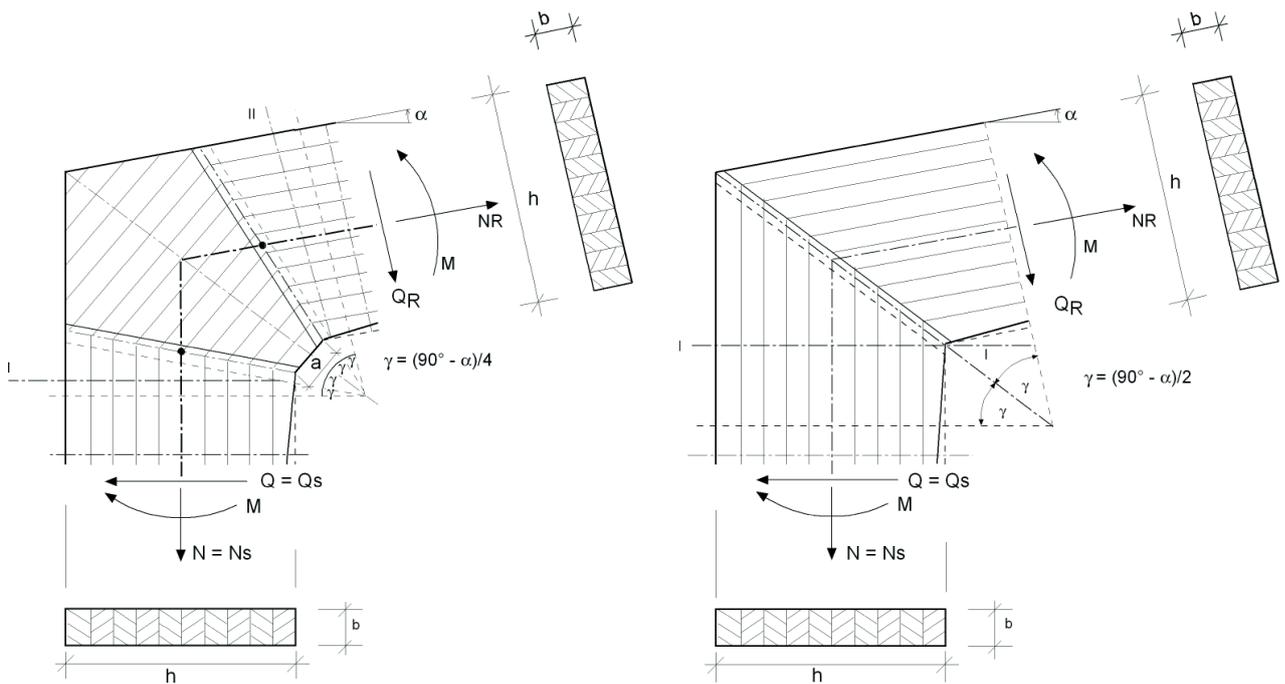
III.: Connection with one or two wedge finger joints.
