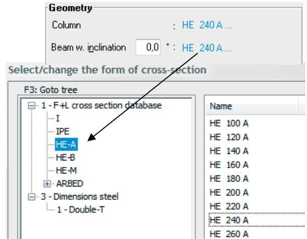
**Beam inclination** angle between the centre line of the beam section and the horizontal line in degrees.
