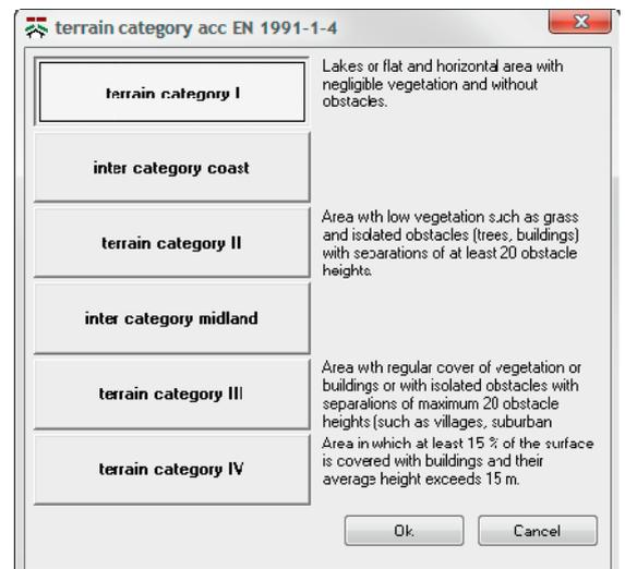
The velocity pressure  $q$  is determined for the maximum building height  $z$  in accordance with EN 1991-1-4, 4.
