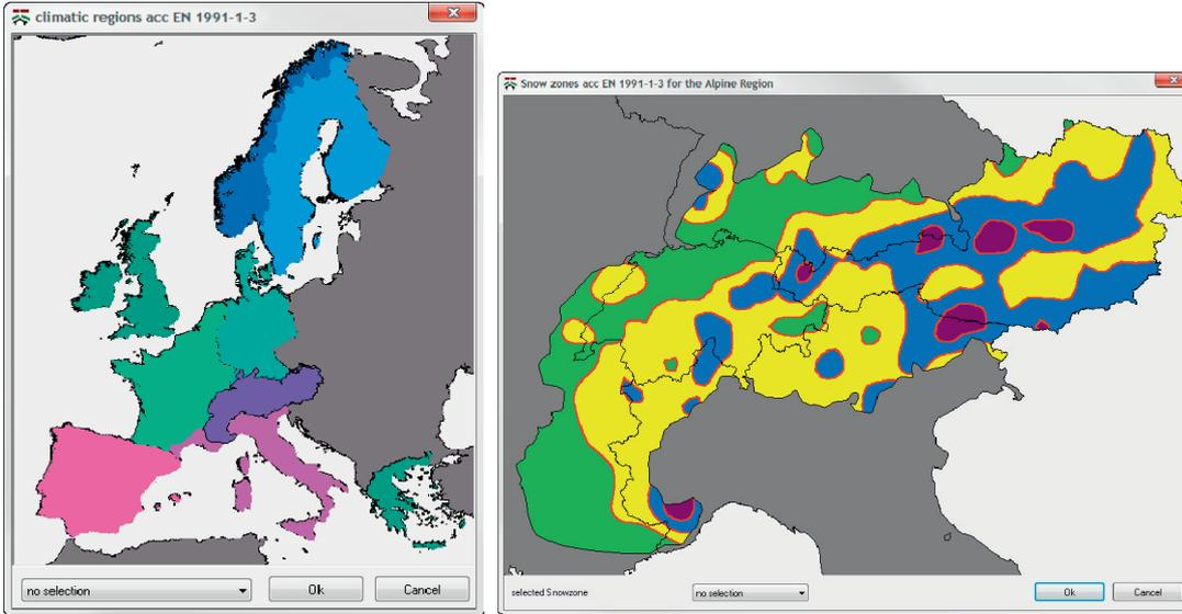
In the associated software applications, the roof snow load  $s_i$  can be calculated with the help of the regular snow load  $s_k$  as follows:
