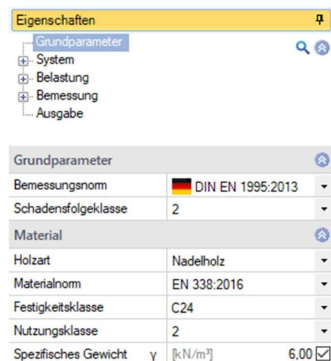
The screenshot shows the 'Eigenschaften' (Properties) window. It contains a tree view on the left with the following items: Grundparameter (selected), System, Belastung, Bemessung, and Ausgabe. Below the tree view is a table for 'Grundparameter' with the following data:
