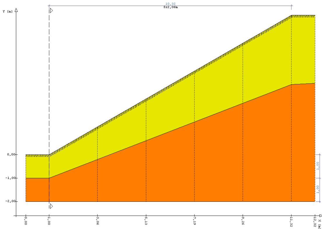
Example 2: the division variant "Number": the distance of 10.32 m is divided into five sections. The resulting section width is 2.06 m
