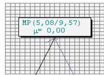
The maximum radii are determined by the soil quantity that was defined. The possible minimum radii are determined by the minimum penetration depth of the slip circles. The minimum penetration depth is defined in the basic parameters.
