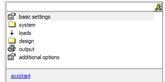
The definition wizard shall facilitate the parameter setting in standard cases. It is often helpful to generate a structural system using the wizard and refine it subsequently with the help of the other available definition functions.
