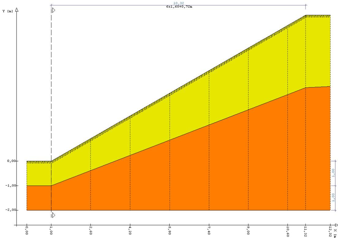
Example 1: the illustrations above and below show the graphic screen and the data-entry field for the division variant "Distance". The distance of 10.32 m length is divided in sections of 1.60 m each. The result is six sections with a length of 1.60 m and a remainder with a length of 72 cm.
