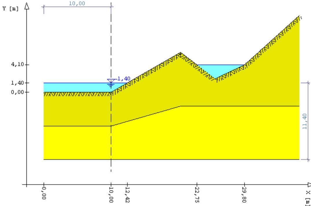
You can define any number of waters (insert...). Water is always determined by a point on the polygon ground surface line and the water depth defined for this point. The banks on the left and right are calculated and the water is shown in the graphical representation. The currently edited water is shown with a section view and the dimensioning.
