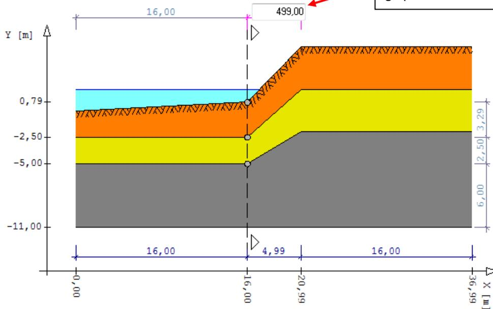
The number of ground profile polygons can be adjusted via the options "Insert", "Delete" and "Delete all".
