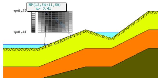
For the calculation of the utilization, the method of slices is used in accordance with BISHOP. The utilization is calculated for a slip circle, which is determined by its centre and its radius.
