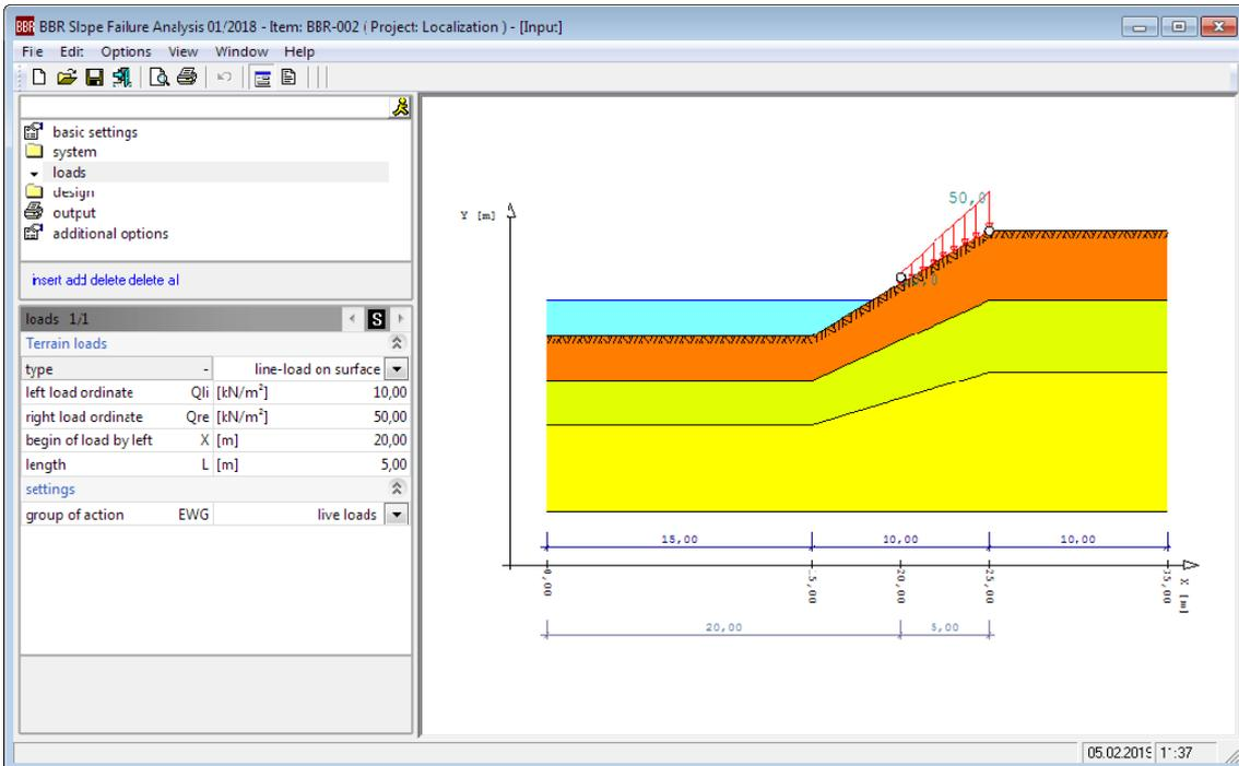
If the mouse cursor is on the data-entry field "Loads", the graphical representation shows the currently edited load always in combination with two circles. You can control the number of loads via the "Insert", "Delete" and "Delete all" options. After completion of the editing process, you are prompted whether to generate an additional load. The currently selected load on the left can be moved in the graphic on the right via the circles shown at the bottom of the load arrow.
