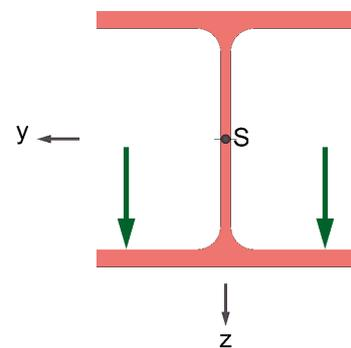
These loads produce secondary flange bending stresses in the proximity of the load application point in two directions. The application calculates the stresses resulting from the local load introduction and superimposes them with the global beam stresses. This local loading can be taken into account in combination for double-T beams with or w/o top flange angles.
