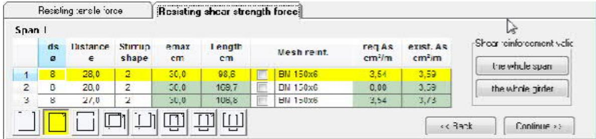
Double-shear and quadruple-shear stirrups and stirrup and fabric meshes are available as reinforcement
