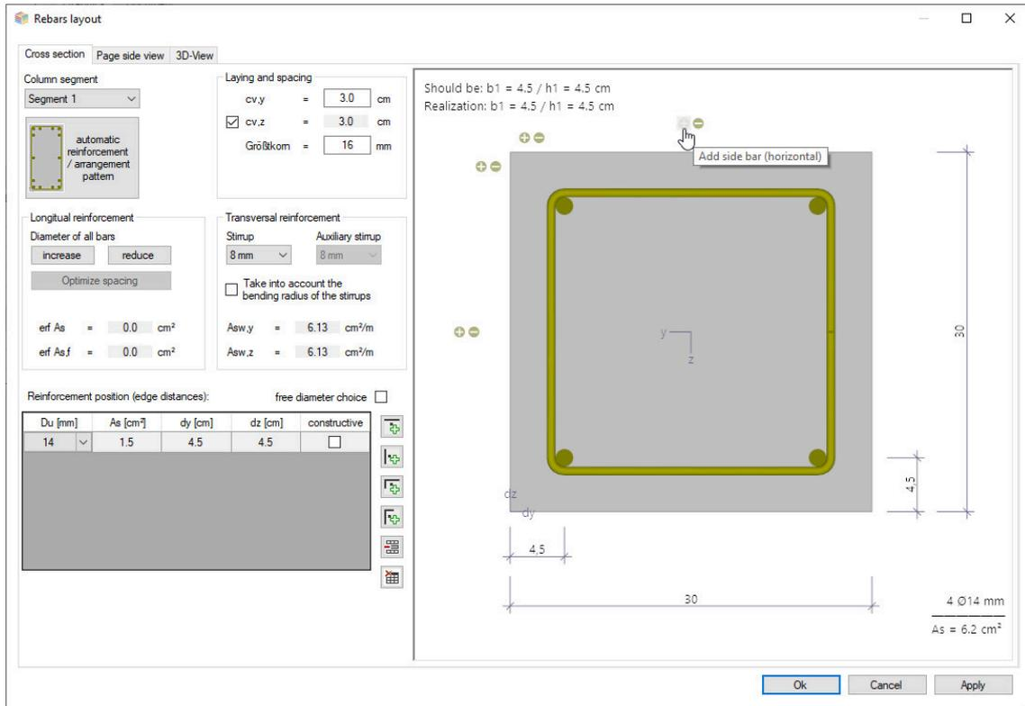
The reinforcement dialog automatically suggests a standard-compliant reinforcement arrangement in the cross-section (incl. necessary structural bars and intermediate stirrups or S-hooks) as well as over the column segment height (with optional consideration of compaction areas).
