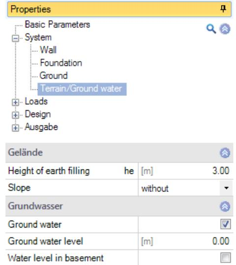
The screenshot shows the 'Properties' dialog box with a tree view on the left containing 'Basic Parameters', 'System', 'Wall', 'Foundation', 'Ground', 'Terrain/Ground water' (selected), 'Loads', 'Design', and 'Ausgabe'. The main area is divided into three sections: 'Gelände' with 'Height of earth filling' (he) set to 3.00 [m] and 'Slope' set to 'without'; 'Grundwasser' with 'Ground water' checked and 'Ground water level' set to 0.00 [m]; and 'Water level in basement' which is unchecked.
