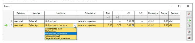
Load type Uniform load, trapezoidal load and point load.
