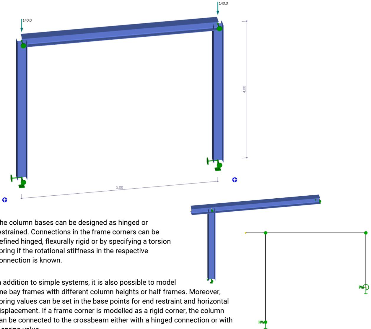
The column bases can be designed as hinged or restrained. Connections in the frame corners can be defined hinged, flexurally rigid or by specifying a torsion spring if the rotational stiffness in the respective connection is known.
