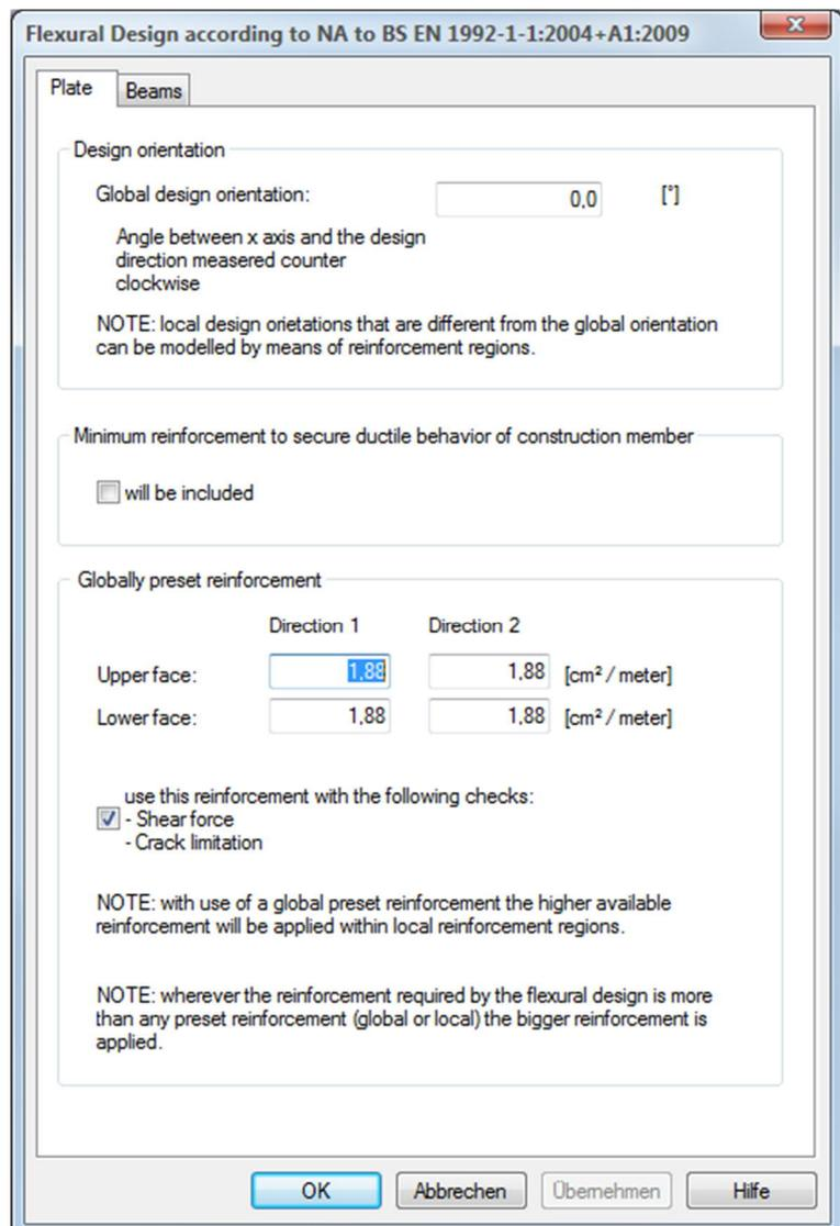
**Flexural Design according to NA to BS EN 1992-1-1:2004+A1:2009**
