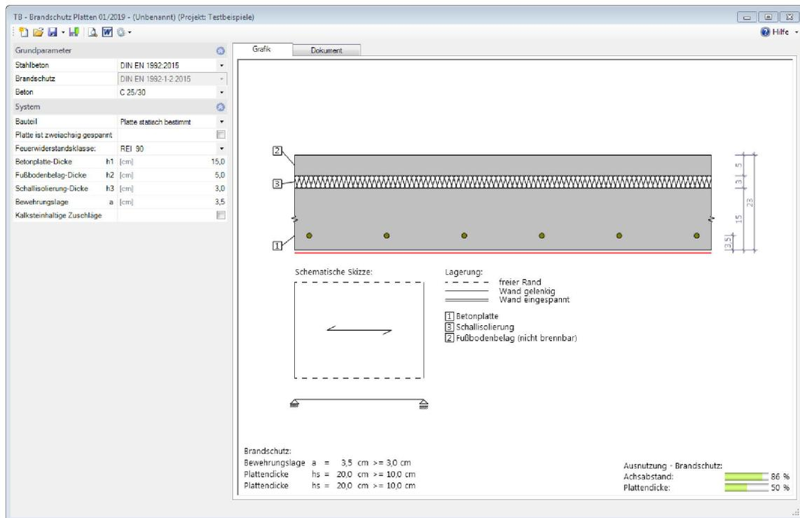
The screenshot displays the TB-BXP software interface for fire protection design. The main window shows a cross-section diagram of a slab with various layers and reinforcement. The diagram includes labels for different components: 1) Betonplatte (concrete slab), 2) Fußbodenbelag (nicht brennbar) (non-combustible floor covering), and 3) Schallsollierung (acoustic insulation). The diagram also shows the reinforcement layout and the slab's thickness.
