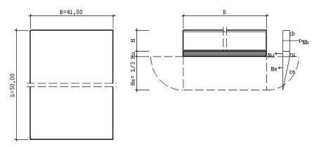
The reactive force is calculated in accordance with /5/ Eq. 6 assuming identical strain in the soil (joint), subconcrete and floor slab:
