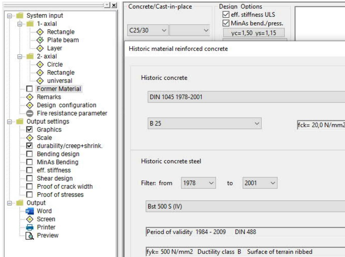
If the option "Former Material" is activated, the standard selection for concrete and reinforcing steel is modified.
