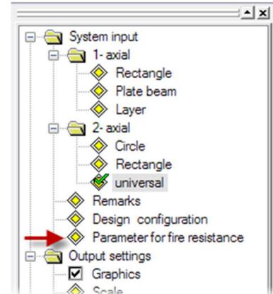
**Fire resistance:** Select a fire-resistance class among R30, R60, R90, R120, R180 according to the target fire-resistance period.
