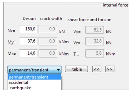
Nx longitudinal force, point of application in accordance with the [Configuration](#), positive tension, negative compression
