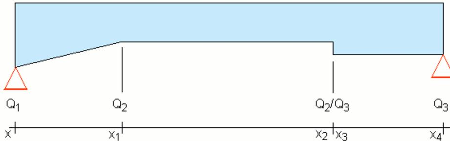
$x$  Distance of the change in cross section to the left support in [m].
