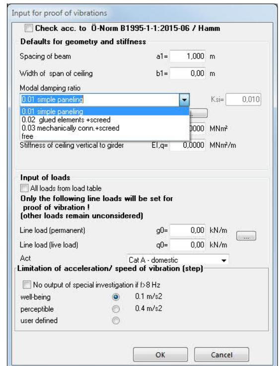
Limitation of the acceleration / speed of vibration (EN 1995)
