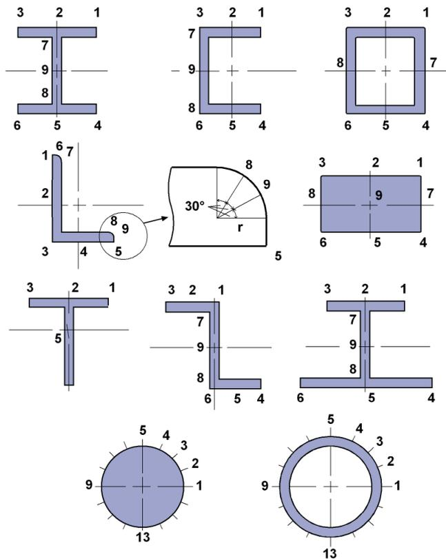
Figure: Profile section overview (Frilo profile selection file) / output points for stresses
