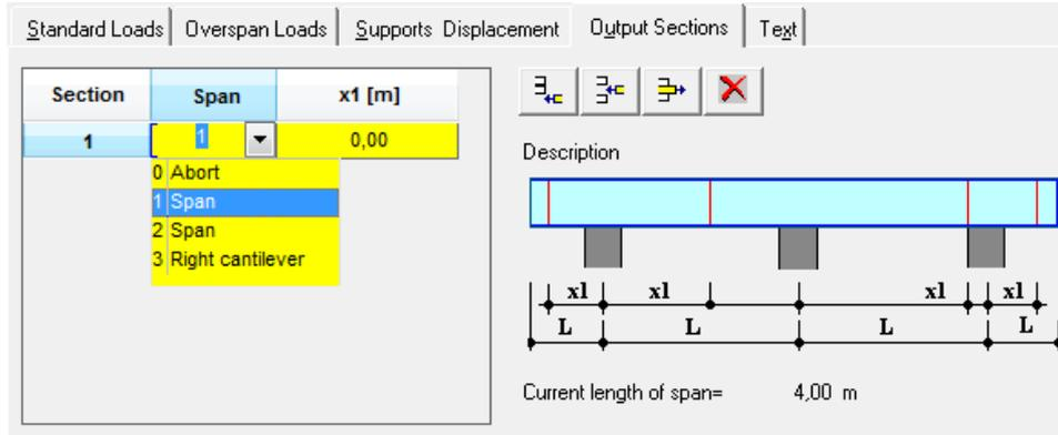
Define sections by entering or selecting a [span number](#) and the distance "x1" to the left support [m]. With left cantilevers, the value refers to the distance to the first (left) support.
