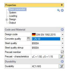
Note: For high-strength concrete (> C50/60), it may be useful to activate the "Design with net Ac"
