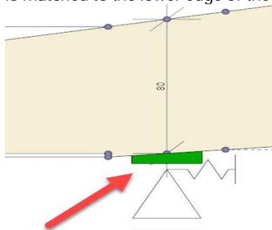
Lx length of the support area in girder direction. It is at most as large as the support area.
