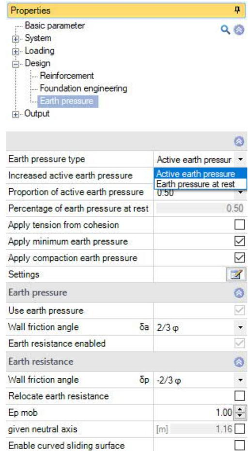
The screenshot shows the 'Properties' dialog box with the 'Earth pressure' section expanded. The settings are as follows:
