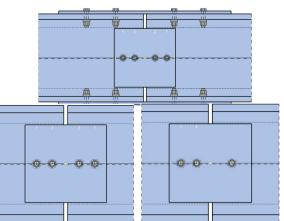
The connection consists of two double symmetrical I-beams that are connected by a bolt connection using a web splice plate on both sides. Different cross-sections can be selected
