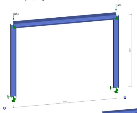
The column bases can be designed as hinged or restrained. Connections in the frame corners can be defined hinged, flexurally rigid or by specifying a torsion spring if the rotational stiffness in the respective connection is known.
