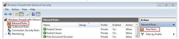
A new port shall be set up and enabled. You can also enable the access to a specific application. This is unsuitable, however, because FRILO offers about ninety standalone software applications.
