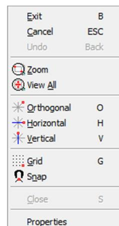
After activating either the "Close" or "Exit" function, the dialog for the definition of the metal plate is displayed. You can enter the plate thickness in mm and the desired "direction of extension" in relation to the defined polygonal chain.
