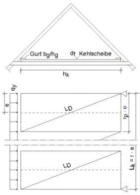
Because of the lack of shear flow all around, the valley plate cannot be calculated like a timber panel according to EN 1995-1-1, 9.2.3 (DIN 1052:2008, 10.6). The valley plate is treated according to the truss analogy, the side planks act as belts, the slab as a substitute diagonal.
