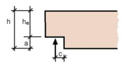
The notch is calculated according to EN 1995-1-1:2008/2014, 6.5.
