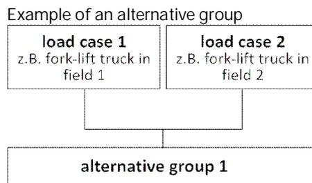
The load cases 1 and 2 are assigned to alternative group 1 because the fork lift is either in field 1 or in field 2.
