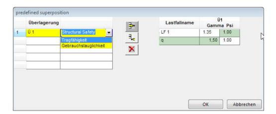
In the left table (superposition) you can specify for each pre-set superposition rule whether a structural safety verification or a serviceability verification is concerned.
