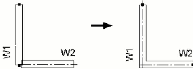
Figure 4: Subsequent point-point connection
