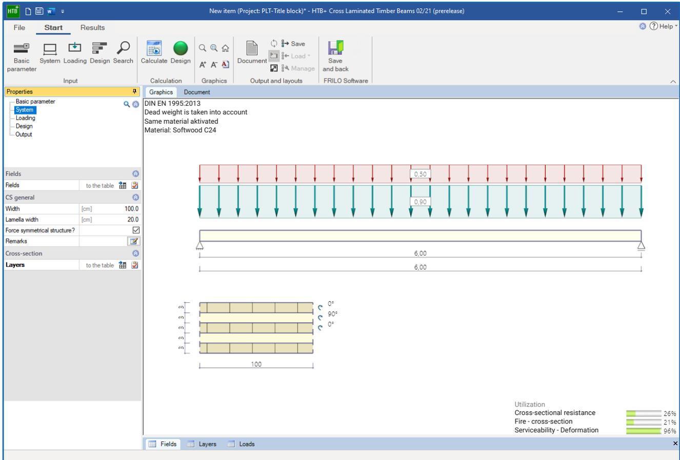
timber glued together at right angles. When entering data, the layer structure can be designed individually with regard to the number of layers, layer thickness and orientation of the layer (lengthways/crossways). In addition, any materials made of softwood or special material parameters from a building authority approval of the cross-laminated timber manufacturer can be entered as user-defined values. In addition, a symmetrical structure can be optionally enforced when entering data.
