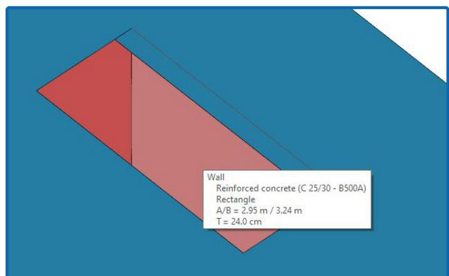
Fig. 9b: A hidden object can be brought into the foreground with the Ctrl key and the scroll wheel - note the tool tip.
