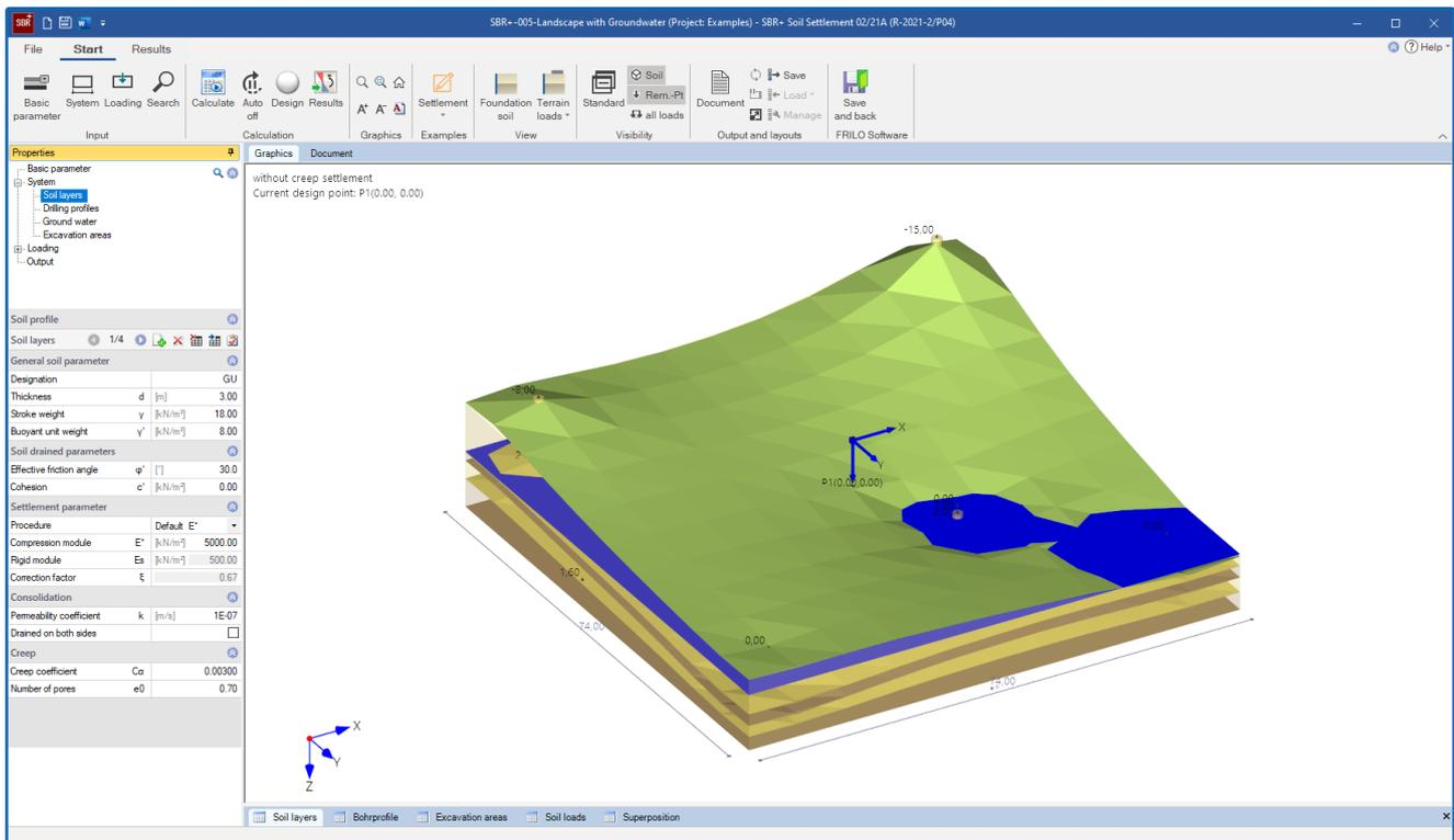
Fig.: The program interface of SBR+ with the new menu items drilling profiles and excavation areas.
