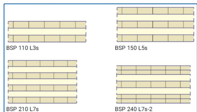
Fig.: Cross-section variants (with manufacturer-neutral designation).
