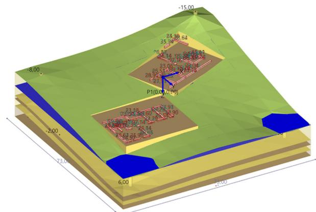
the time course of settlement and foundation tilting caused by changes in the volume or shape of the subsoil. In this calculation, the external loads can be modeled in the form of infinite area loads, arbitrarily positioned limited block loads or asymmetrical trapezoidal loads. The number of terrain loads, their type of action as well as the limit state to be considered and the design situation can be selected as required.
